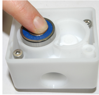
Fig. 9: Press in the driving shaft
