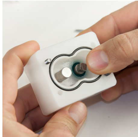
Fig. 5: Press out the driving shaft
