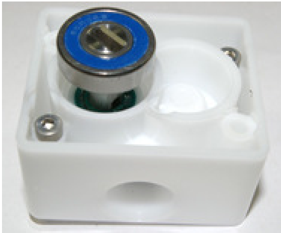
Fig. 6: Remove the driving shaft
