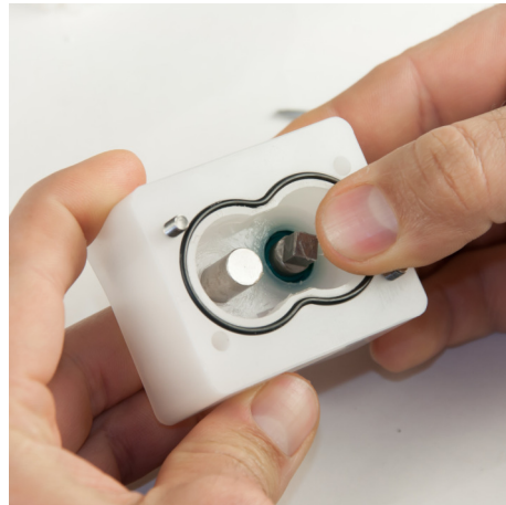
Fig. 6: Press out the driving shaft
