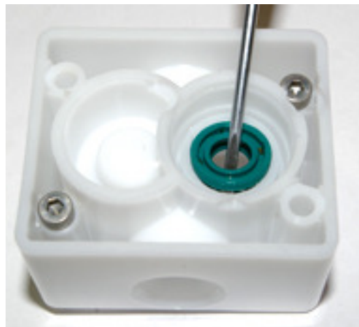
Fig. 8: Remove the shaft seals
